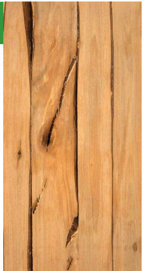
Fig. 1. Longitudinal surface of a glued up Vaccinium corymbosum wood specimen. Wood grown in a plantation in the Netherlands
