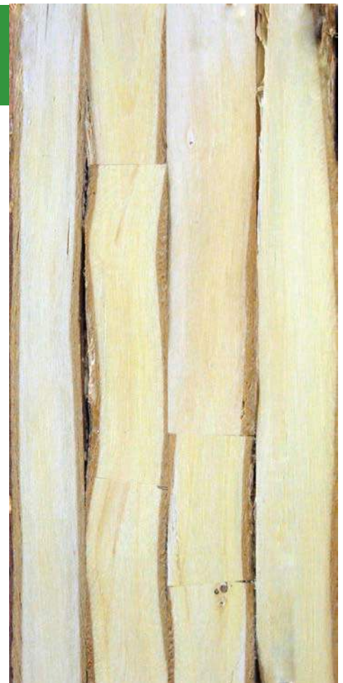
Fig. 2. Longitudinal flat sawn surface of a glued up Passiflora caerulea wood specimen, the wood grown in Crete, Greece
