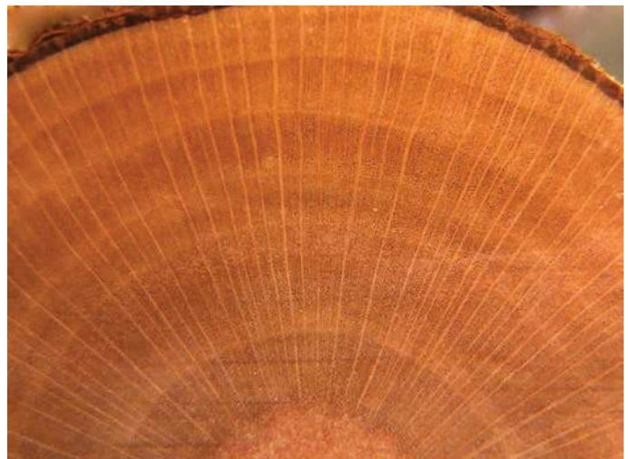
Fig. 3. Lens view (8x) of Vaccinium corymbosum wood endgrain
