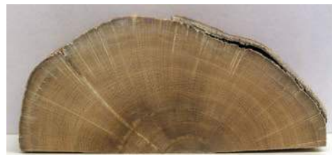
Fig. 5. Transverse surface of an almost half disc of Cestrum parqui stem wood. The diameter of this stem was 8 cm (3.2 in.).
