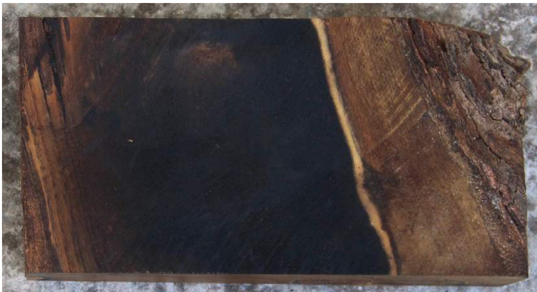
Fig 4. Pistacia terebinthus L. Note pale part of outer heartwood. - Photo by Willem Hurkmans
