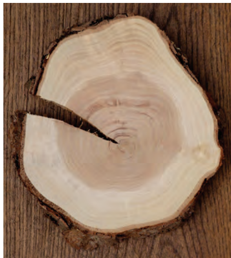
Fig. 9. Dry disc of Nothofagus antarctica near the stem base. Diameter 16 x 18 cm (6.4 x 7.2 in.). Wood collected in the Netherlands.
