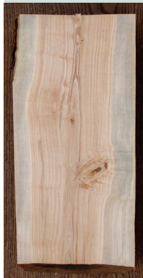
Fig. 8. Dry longitudinal surface, cut and planed over the pith. The length of this piece is little over 30 cm (1 ft.). Wood collected in the Netherlands.
