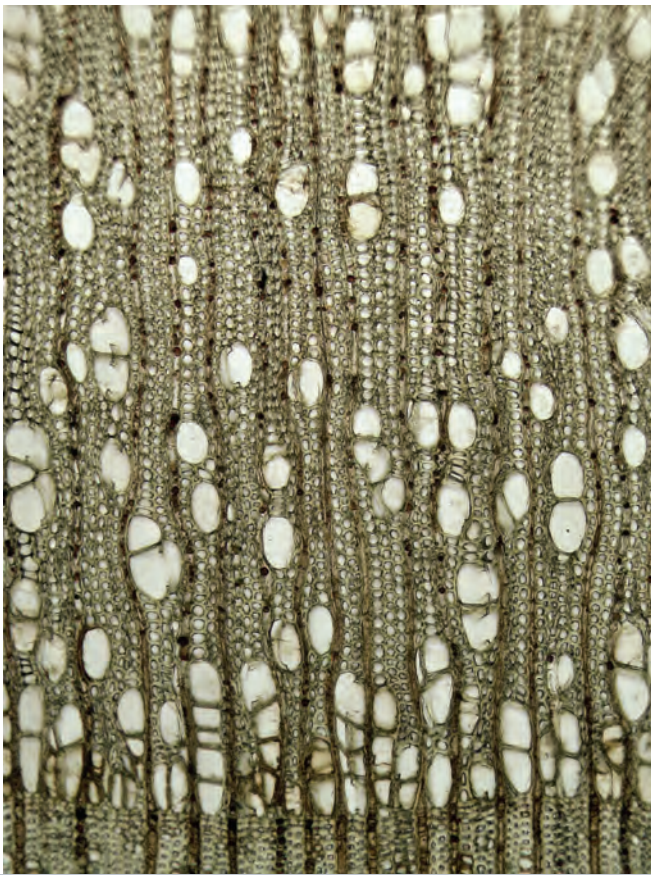
Fig. 12. Photomicrograph (100x) of the cross section of Nothofagus antarctica . Clear, compound ring of earlywood vessels of the same tangential diameter as in the latewood. Photo by Raimund Aichbauer.
