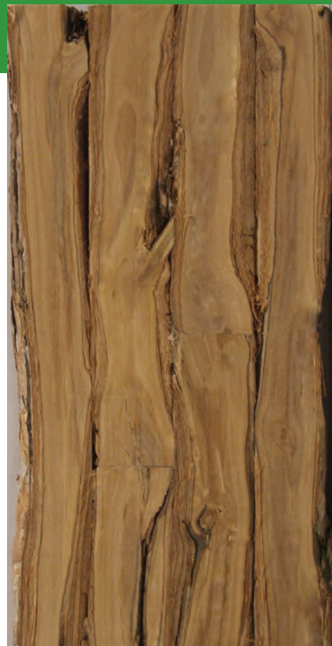
Fig. 1. Longitudinal surface of a glued up Zenobia pulverulenta wood specimen, 2¾ in. (7 cm) wide. The wood was collected in the Netherlands from a small shrub.
